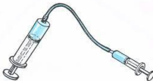
Figure 3 Illustration on how pressure transmit in an enclosed fluid using simple syringe
